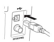
Communication interface in this instrument conforms to USB1.1. Hold the USB cable plug in unplugging. Do not pull the cord. Plug the USB cable to fit the connector entry point.
